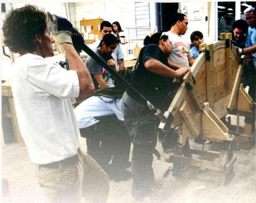
Working with apprentices at Rocking the Boat in Bronx, New York, Geoff McKonly uses a pry bar to persuade a steamed and kerfed stem to conform to a bending jig. The apprentices will not only build a whaleboat but also sail it from New York to Mystic, Connecticut.
